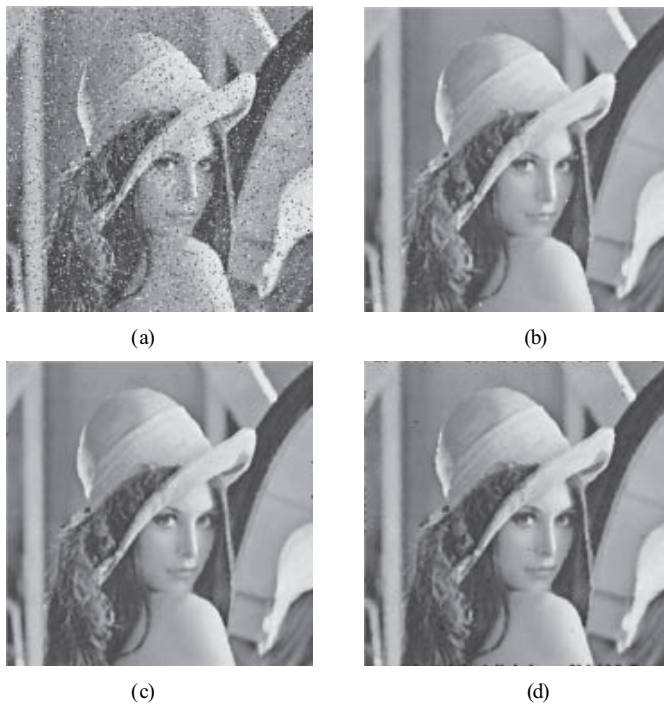
Fig. 41. Simulation results of a 2-D ROF application. (a) The noisy “Lena” image corrupted by 8% of impulsive noise. (b) The “Lena” image processed by the 3 \times 3 4th-order filtering. (c) The “Lena” image processed by the 3 \times 3 5th-order filtering. (d) The “Lena” image processed by the 3 \times 3 6th-order filtering.
